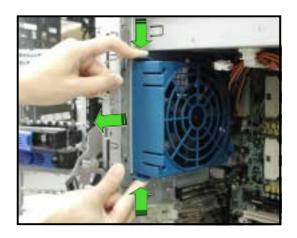
To re-install the chassis fan:
